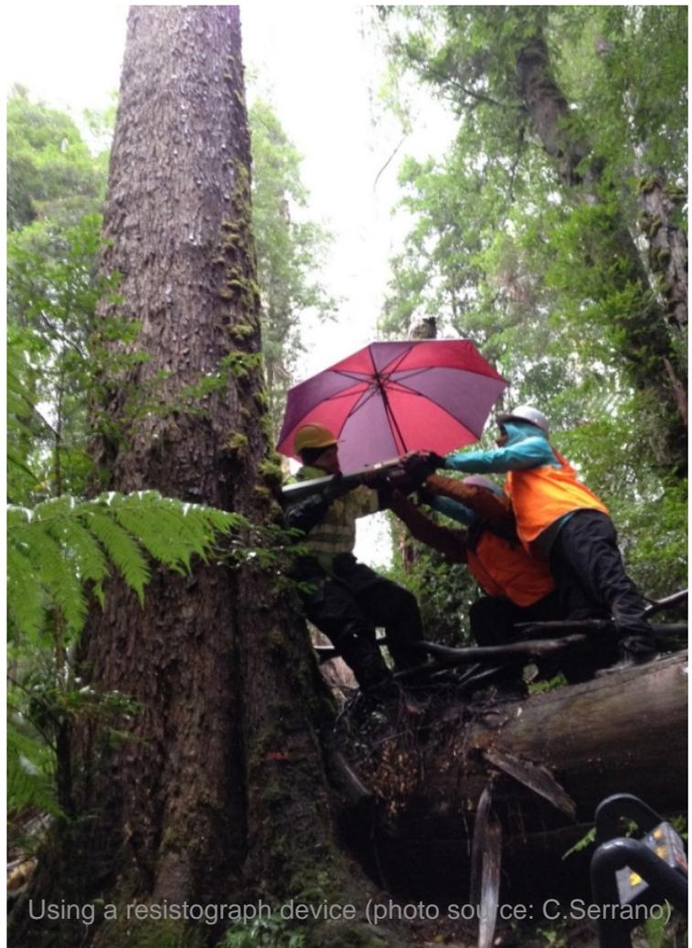
Using a resistograph device (photo source: C.Serrano)
